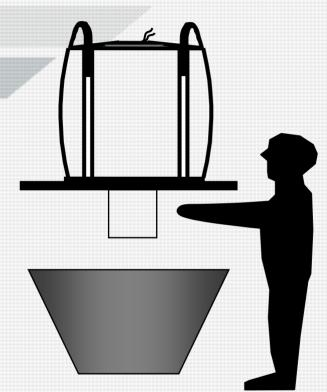
The bottom discharge spout should be opened only when the FIBC is suspended over a Safety support which will prevent injury to the operator in the event of a failure of the lifting device.
