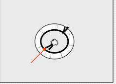
Pull spout down, free of spout cover. Align spout over the receiving device. Pull both ends of the spout tie in opposite directions, gravity will start the flow of the product.
