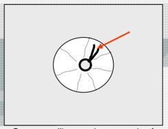
Operator will grasp the two ends of the spout cover ties and pull in opposite directions. Open cover to release spout.
